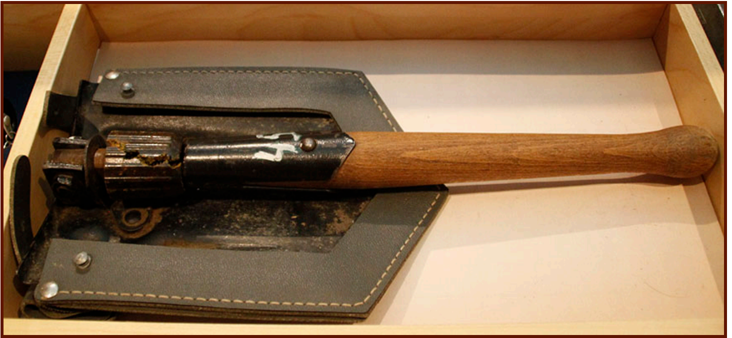
Entrenching Tool – Collapsible shovel strapped to rucksack; used to dig trenches.
